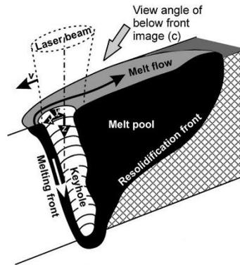
Fig. 1. Sketch of laser beam, keyhole and melt pool, Kaplan (2012).
