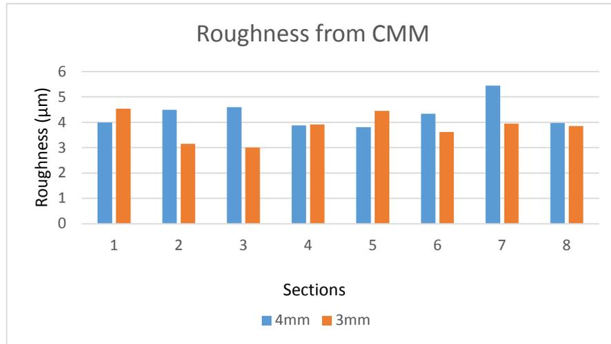
**Figure 7** The  $R_z$  from the CMM machine measurement
