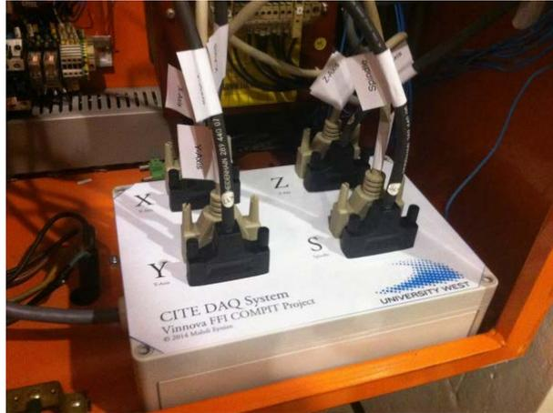
**Figure 4** The CITE hardware for data acquisition, inside CNC machine's control cabinet (source: [15], used with permission)
