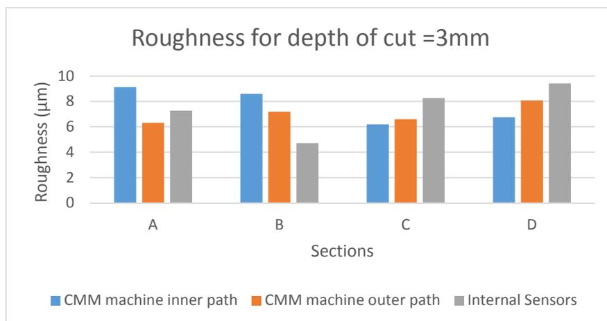
**Figure 10** The  $R_z$  for depth of cut equal to 3 mm
