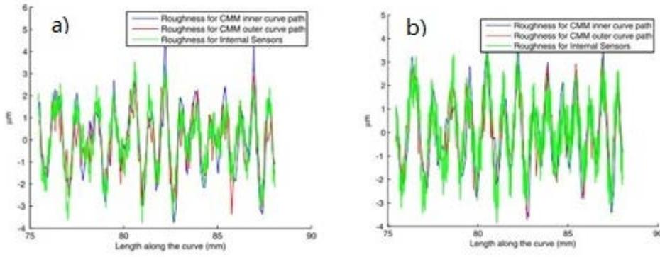
**Figure 11 a)** The roughness for depth of cut equal to 3 mm **b)** The roughness for depth of cut equal to 4 mm
