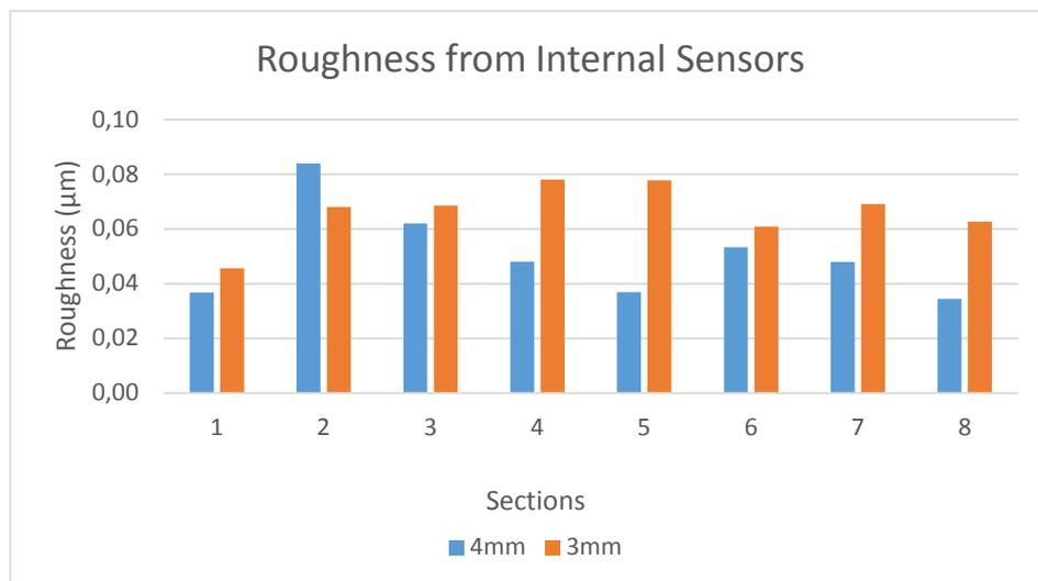
**Figure 6** The  $R_z$  from the internal sensors measurement
