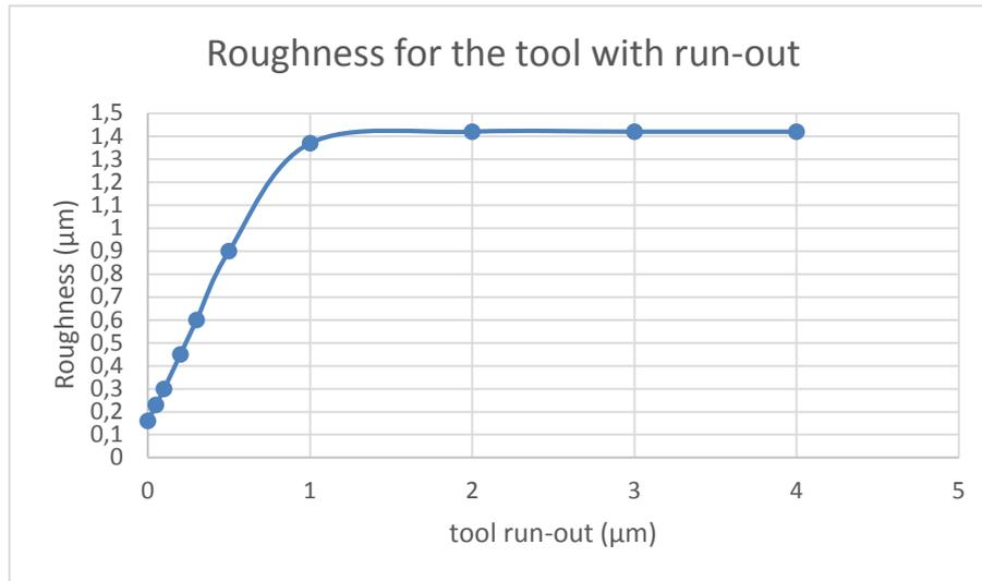
**Figure 13** Roughness for the tool with run-out
