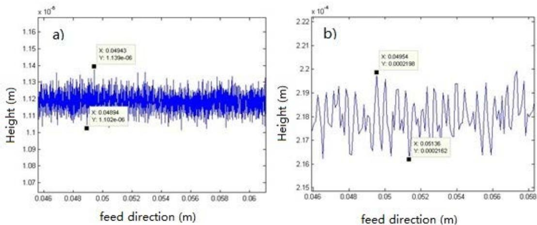
**Figure 8 a)** The small samples in internal sensors measurement errors **b)** The small samples in CMM machine measurement errors
