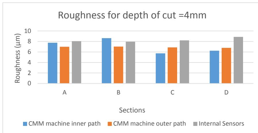
**Figure 9** The  $R_z$  for depth of cut equal to 4 mm
