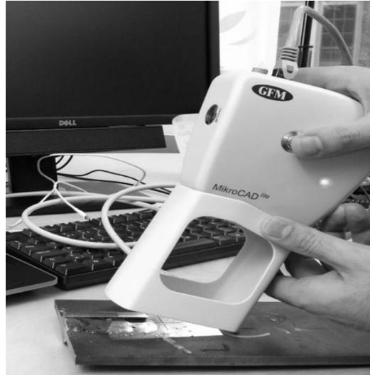
Fig. 4. Measurement setup of Structured Light Projection (SLP) method for measuring the weld toe radius.
