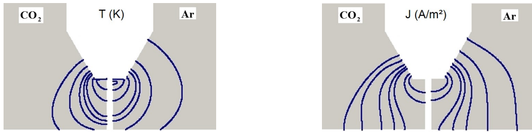
Fig. 4. Zoom of contours between electrode and base metal. Left: temperature T and Right: current density J (with \text{CO}_2 in each left section, Ar in right section). From large to small radius the T -contours (resp. J -contours) correspond to 12, 14, 16, 18, 20, 22 and 24 kK (resp. 1, 2.5, 5, 7.5, 10, 25, and 50 \text{MA/m}^2 ).
