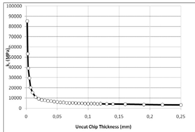
*Figure 7. The  $k_c$  curve extracted from turning Inconel 718 at a cutting speed of  $v_c=50\text{m/min}$ .*
