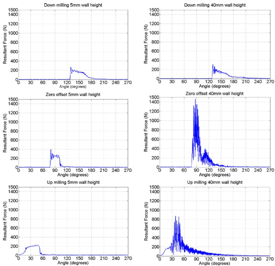
**Figure 5.** Example graphs from the plots in Figure 4. Resultant force measurements for down milling (top), zero offset milling (middle), and up milling (bottom) at 5mm (left) and 40mm (right) wall height overhang.
