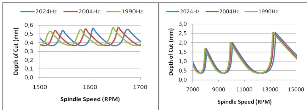
**Figure 2.** Stability Lobe Diagram at the beginning (1990Hz), at the middle (2004Hz), and at the end (2024Hz) of the cut for low speed (left) and high speed (right) milling. Data recorded at low spindle speeds (left graph) and high spindle speed (right graph).
