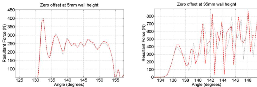
**Figure 6.** Two subsequent force measurements: on left in phase depicting forced vibrations, and on right out of phase depicting chatter vibrations.
