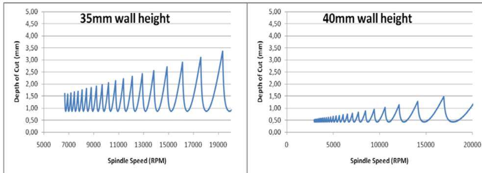
**Figure 3.** The effect on  $a_{lim}$  as the wall height overhang is increased from 35mm to 40mm. The diagrams are experimentally derived from hammer impact tests. As  $a_{lim}$  goes below  $a_p=0.5\text{mm}$ , chatter vibrations are unavoidable.
