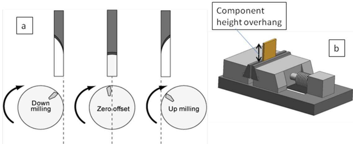
**Figure 1.** a: Top view of the offset positions used in this study. b: Clamping of workpiece.
