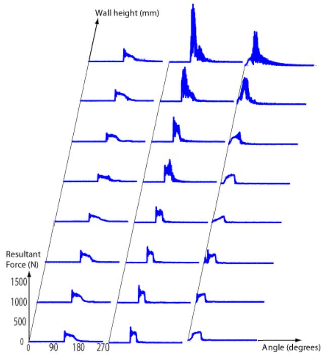
**Figure 4.** Down milling (left), zero offset milling (middle), and up milling (right) at 5, 10, 15, 20, 25, 30, 35, and 40mm (from bottom to top) wall height overhang.
