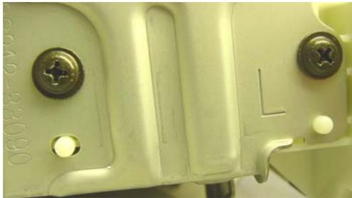
Figure 26: Screw joint and locator pins from Toyota Lexus. The circular hole guides the part in the x- and z-direction. The oval hole guides in the z-direction and may compensate for difference of the tolerances in the x-direction. This concept may reduce the risk of tensions.
