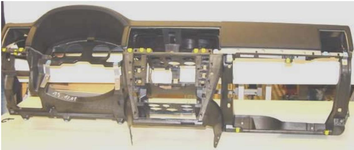
**Figure 4: The radio carrier is integrated into the panel carrier by welding. The centre stack area has high stiffness and the parts are well attached in separated sections.**
