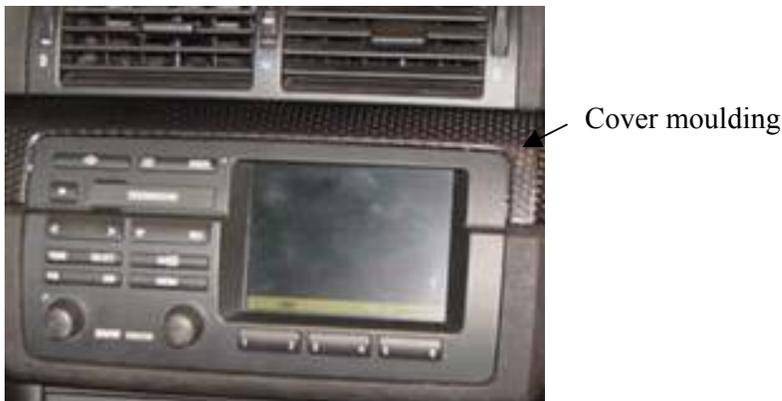
**Figure 8: The problem with screw joint is to find suitable attachment points and how to conceal them. The concept with cover moulding makes it easier to use screw joint.**
