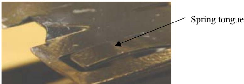
**Figure 13:** To get preload in the z-direction, a spring tongue may be used. The radio tightens the spring tongues that provide a preload between the radio carrier and the sleeve.
