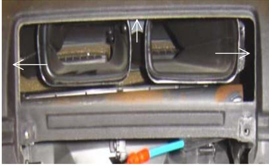
**Figure 18: Contact surfaces for the air outlet.**
