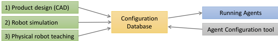
Figure. 3. This figure shows the agent configuration tool together with some additional supporting tools 1,2 and 3. All these four tools can be connected to the agent configuration database and automatically deployed to agents in the manufacturing system.
