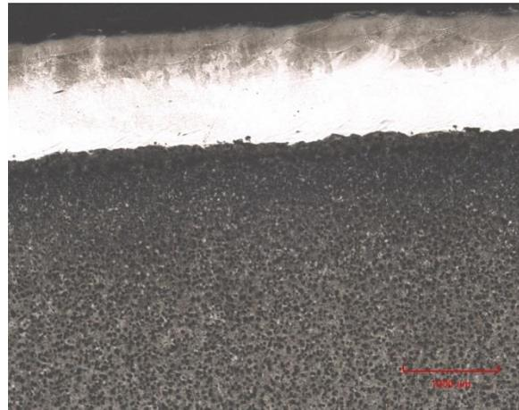
*Figure 5, general picture of a sand blasted surface with 1 layer of SS sample.*
