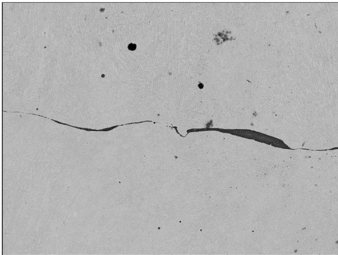
Figure 30, SEM of voids and crack in a grit blasted specimen with 2 SS layers
