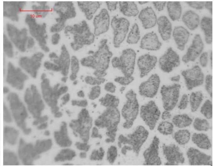
Figure 14, inter-layer area of a buffered specimen with 1 SS layer
