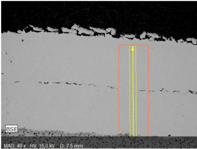
Figure 34, position of the EDS line scan on a machined specimen with 2 SS layers
