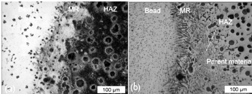
*Figure 1, Optical Images of ductile cast iron welded with a 57.2% Ni-Fe electrode [5]:*
