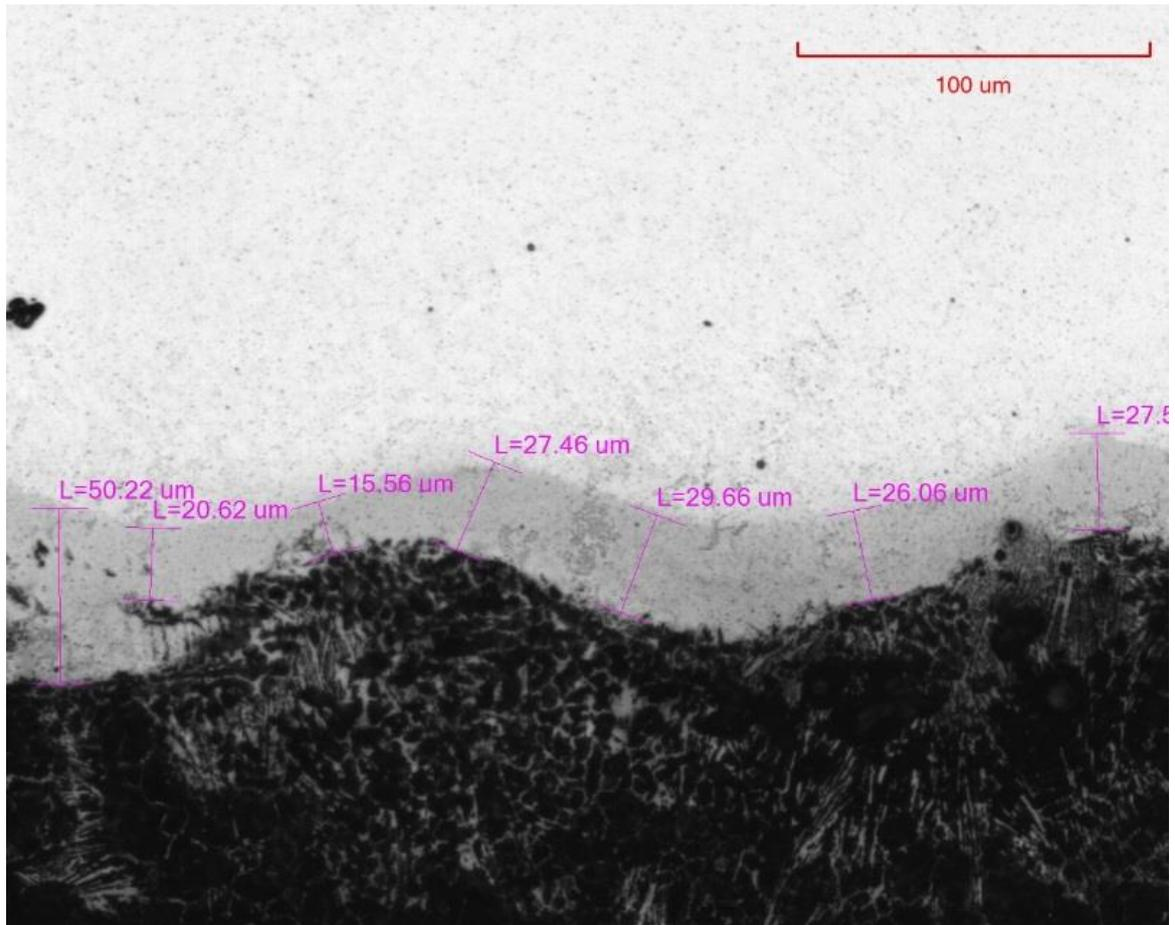
*Figure 6, substrate-coating interphase of a grit blasted sample with 2 SS layers*
