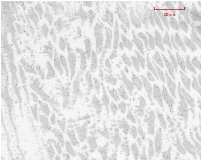
Figure 12, inter-layer area of a grit blasted specimen with 2 SS layers
