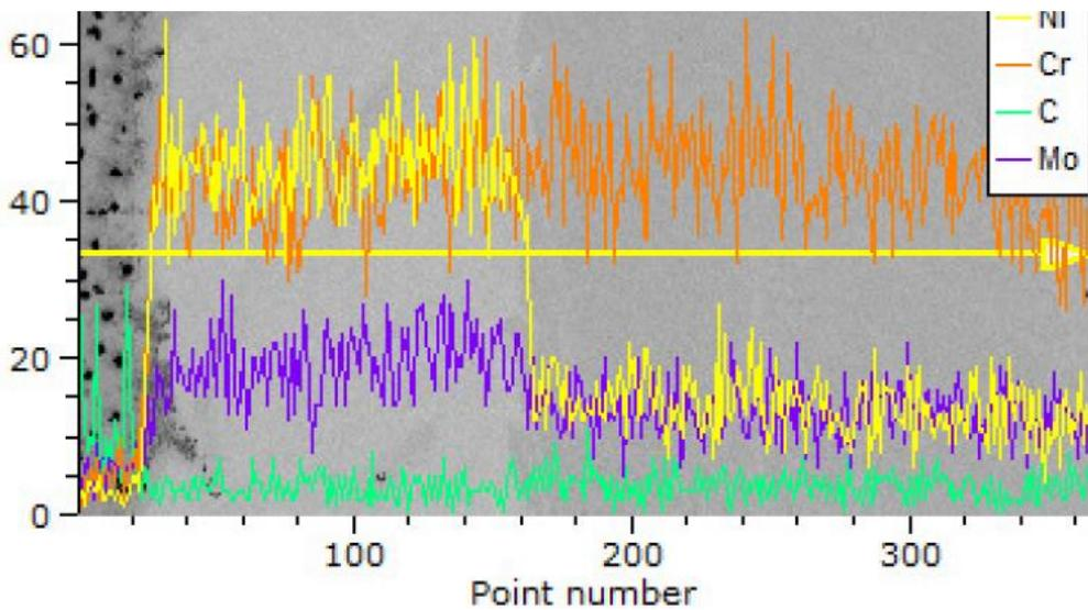
Figure 37, results of the EDS line scan on a buffered specimen with 1 SS layer
