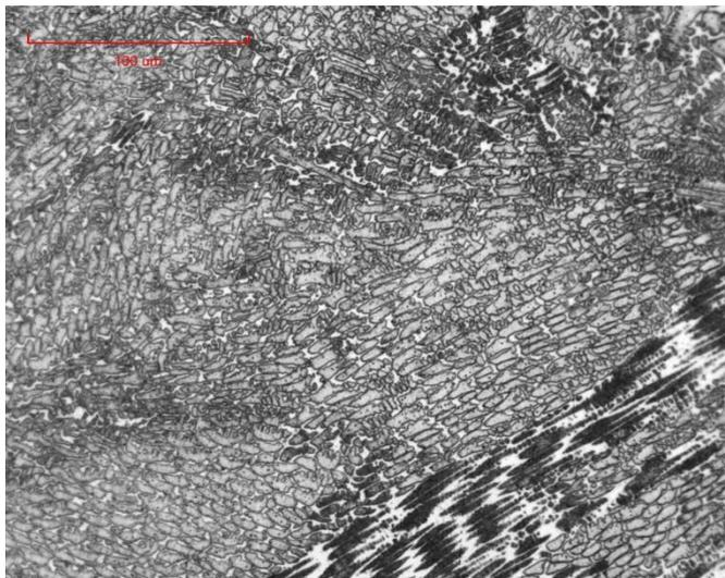
*Figure 19, surface area of a machined specimen with 3 SS layers*
