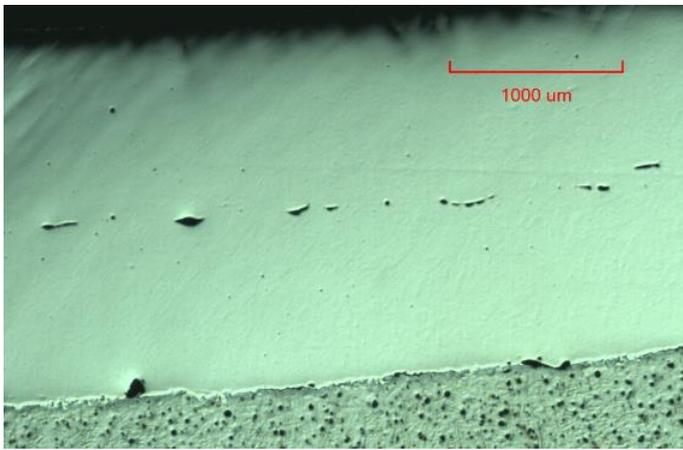
Figure 28, voids and crack in a grit blasted specimen with 2 SS layers
