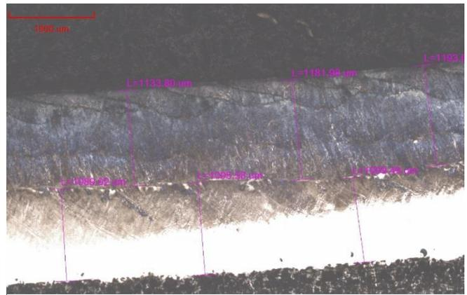
*Figure 8, layer thickness of a surface remelted machined sample with 2 SS layers
