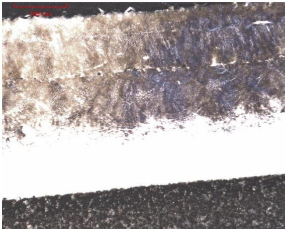
*Figure 4, general picture of a machined surface with 3 layers of SS sample.*
