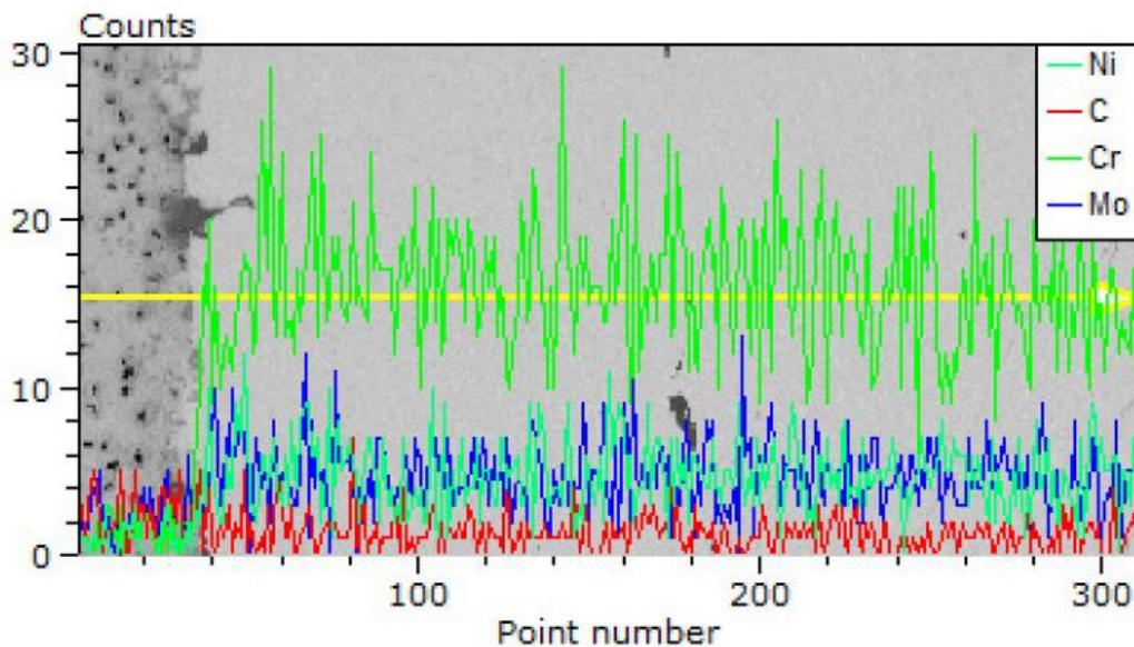
Figure 33, results of the EDS line scan on a grit blasted specimen with 2 SS layers
