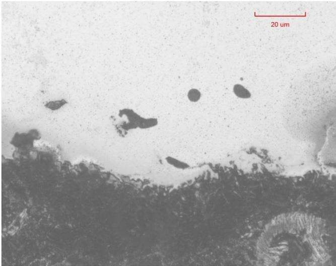
Figure 11, substrate-coating area of a grit blasted specimen with 2 SS layers
