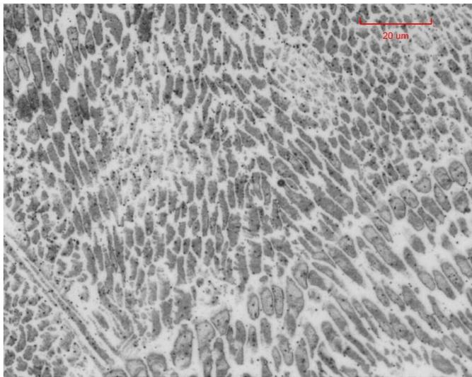
Figure 13, surface area of a grit blasted specimen with 2 SS layers
