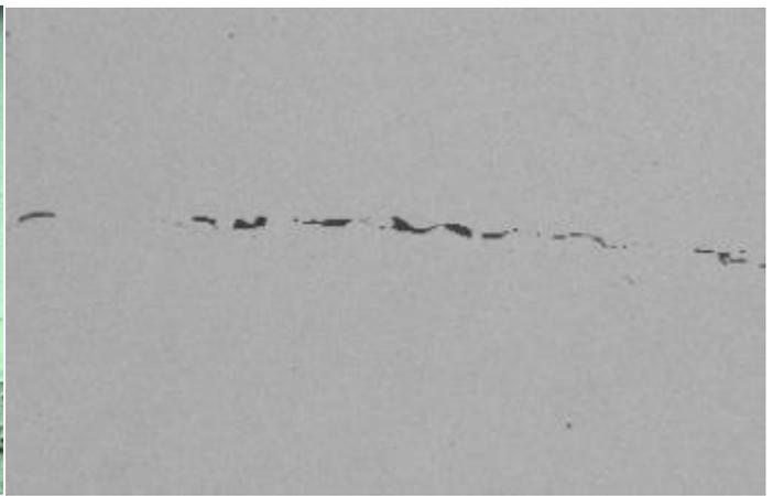
Figure 29, SEM of voids and crack in a machined specimen with 2 SS layers
