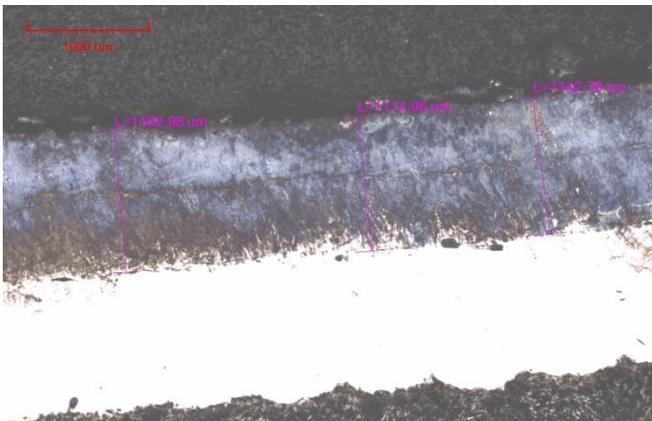
*Figure 7, layer thickness of a machined sample with 2 SS layers
