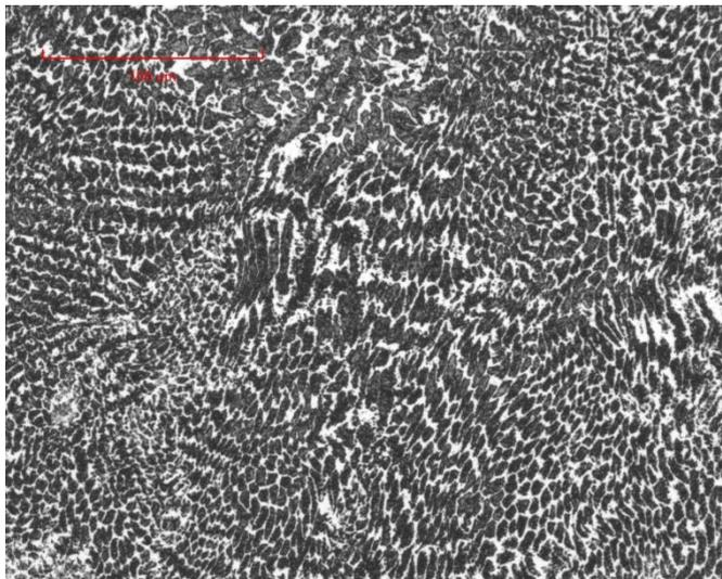
*Figure 18, surface area of a buffered specimen with 2 SS layers*
