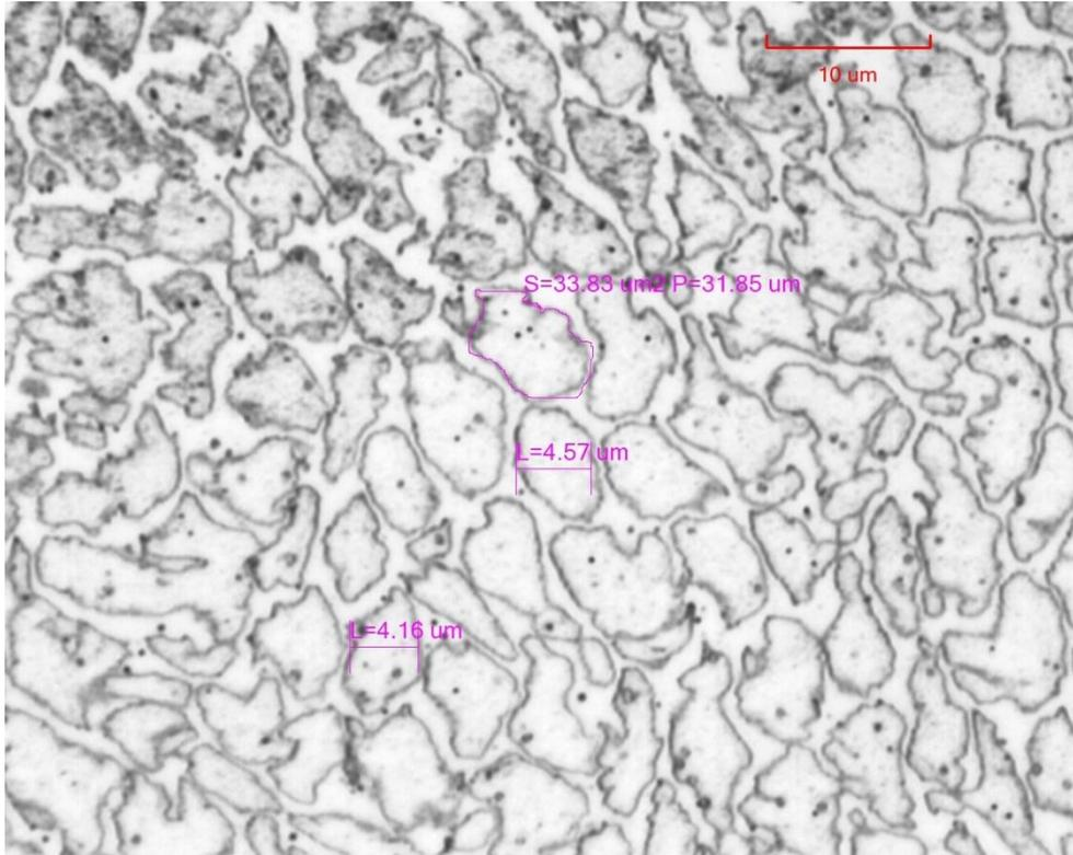
Figure 22, direct cell size measurements of the surface area of a machined specimen with 1 SS layers
