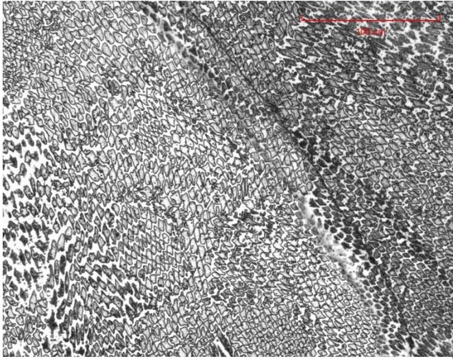
*Figure 17, surface area of a grit blasted specimen with 3 SS layers*
