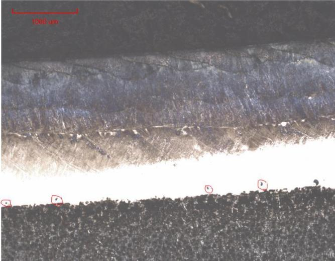
Figure 26 detected voids in a machined and remelted specimen with 2 SS
