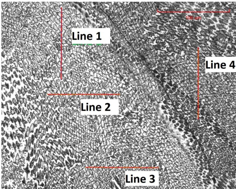
Figure 25, ASTM Intercept Method cell size measurements on the surface area of a grit blasted specimen with 3 SS layers
