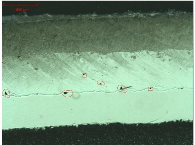
Figure 27, detected voids in a buffered specimen with 2 SS layers
