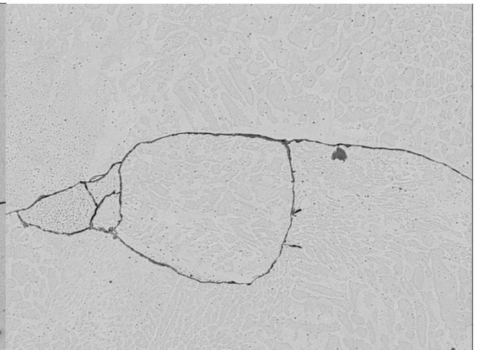
Figure 31, SEM of voids and crack in a machined specimen with 2 SS layers
