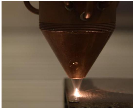
*Figure 2, Coaxial LMPD feeding nozzle used in the project*
