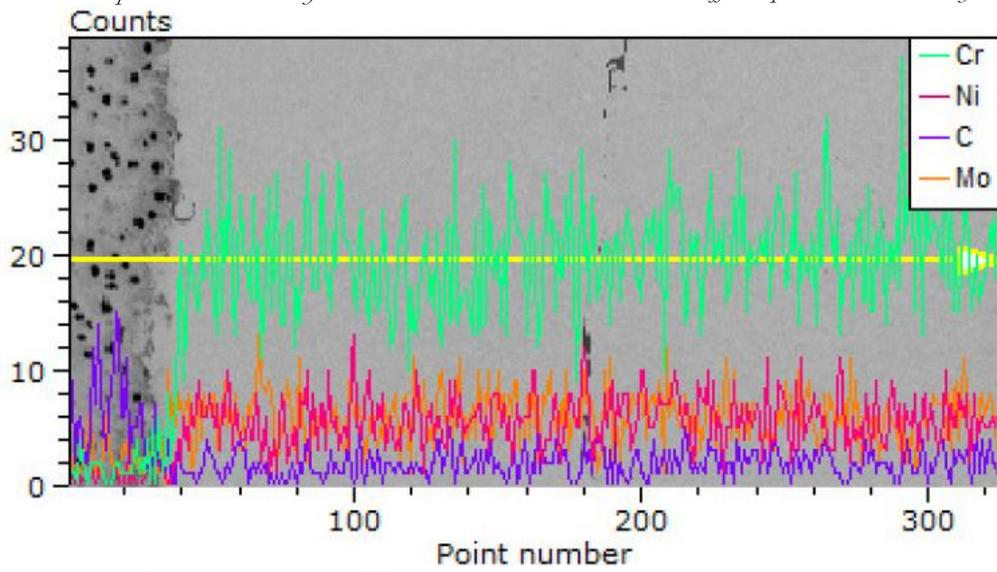
Figure 35, results of the EDS line scan on a machined specimen with 2 SS layers
