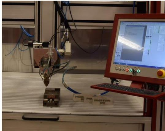
*Figure 3, Robotized LMPD system*
