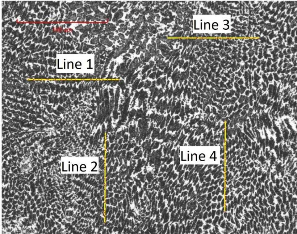
Figure 24, ASTM Intercept Method cell size measurements on the surface area of a buffered specimen with 2 SS layers
