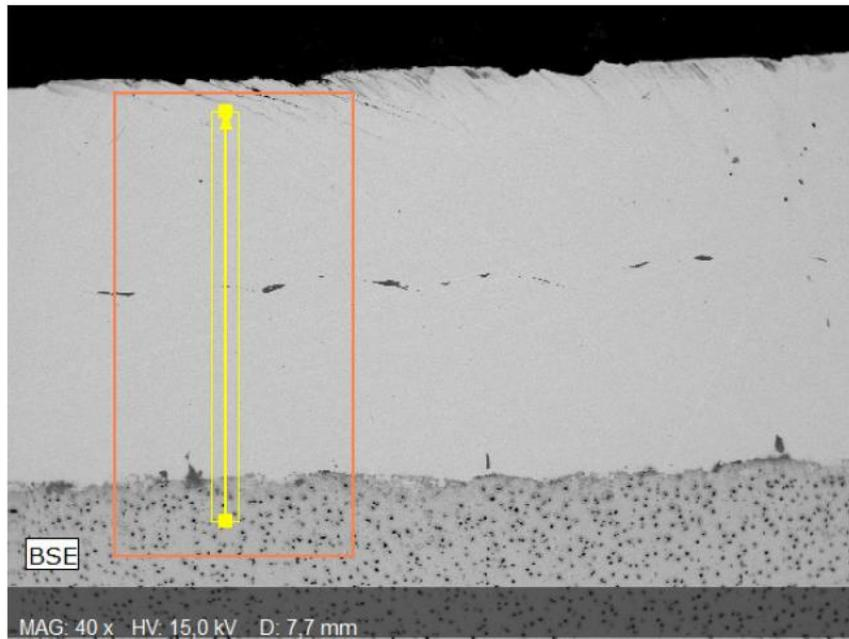
Figure 22, position of the EDS line scan on a grit blasted specimen with 2 SS layers
