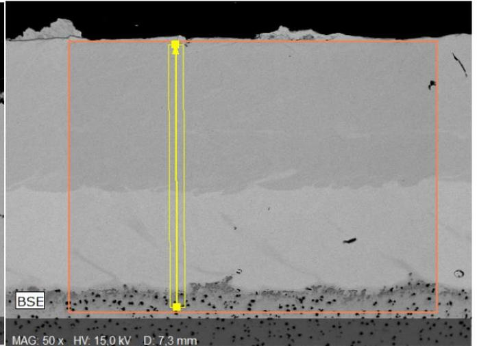
Figure 36, position of the EDS line scan on a buffered specimen with 1 SS layer
