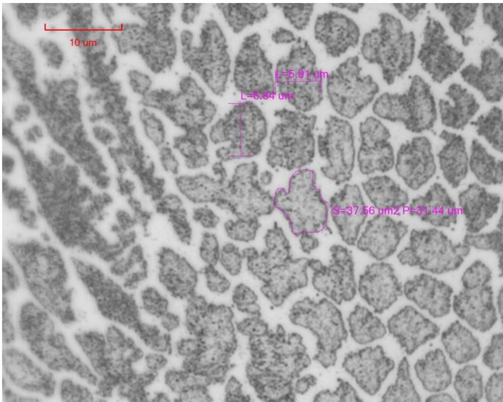
Figure 23, direct cell size measurements of the surface area of a machined specimen with 3 SS layers
