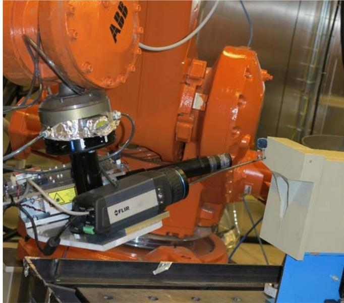
**Fig. 3.** The inspection cell with the measuring head mounted on a six axes industrial robot. The mock-up, shown at the right in the picture, resembles inspection of a jet-engine component with limited access.
