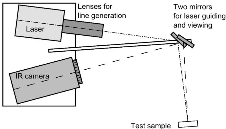
**Fig. 1.** Measuring head for inspection of surface cracks in welds with limited access.
