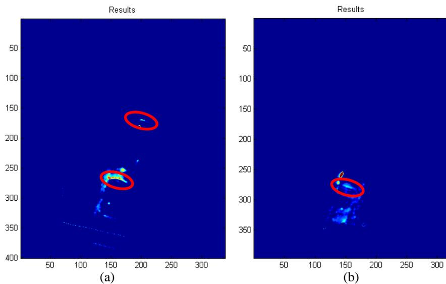
**Fig. 7.** Thermography results for (a) test sample 4 and (b) test sample 9. Real cracks detected by the analysis are marked with rings
