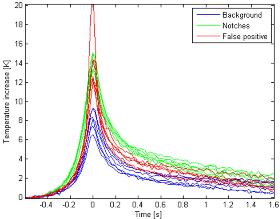
Fig. 2. Temperature increase in several notches, background points and false positives.
