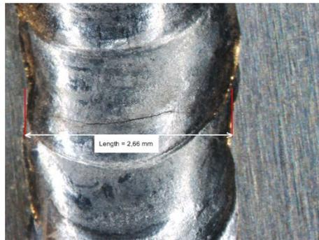
**Fig. 6.** The crack across the weld in test sample 9.
