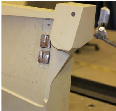
**Fig. 4.** The open mock-up with the welded test plates visible. The upper test sample is named “sample 4” and the lower “sample 9”.
