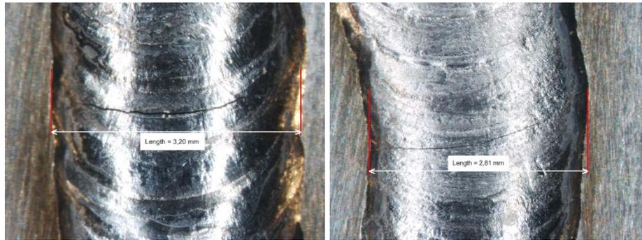
**Fig. 5.** Two cracks across the weld in test sample 4.
