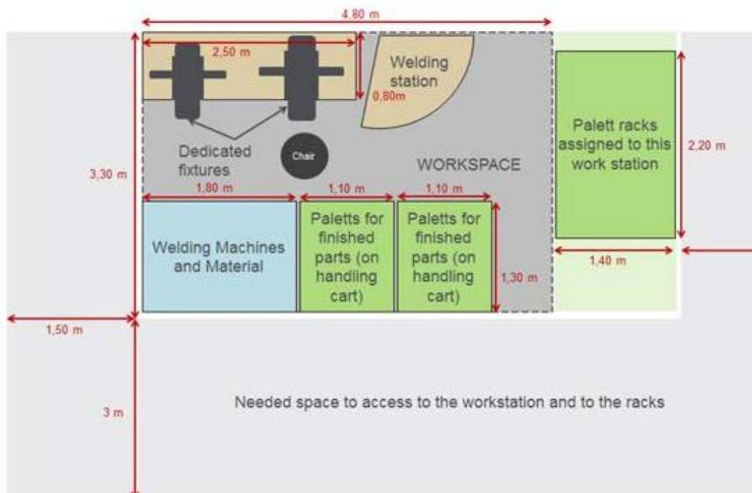
**Figure 2.** The layout of the current workstation, made by Ferry Clément and Le Pol Martin Vincent from VCE.
