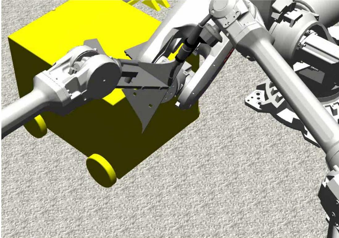
**Figure 4.** Automatic assembly and tack welding
